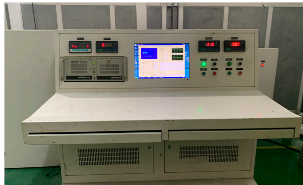
Fan performance test data acquisition system
