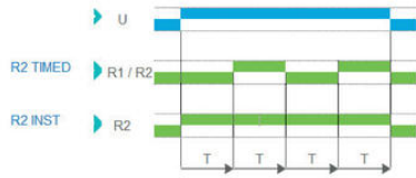
Function D - Symmetrical flashing (OFF Start)
