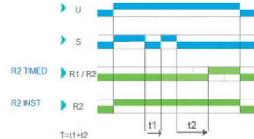
Function At - Summation time relay
