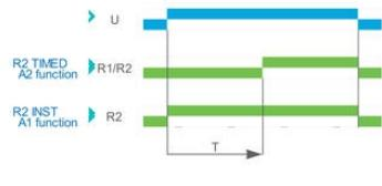
Function Ac - On/Off Delay (Delay on make/break)
