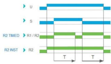
Function C - Off-Delay (Delay on break)
