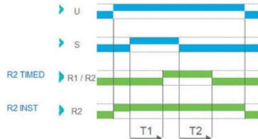
Function Ac - On/Off Delay (Delay on make/break)
