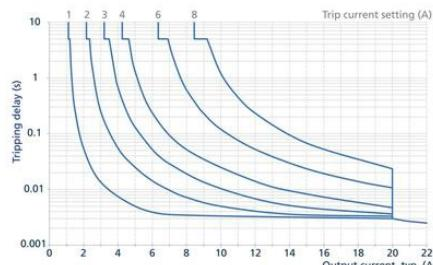
Fig. 6-2: Tripping delay depending on current
