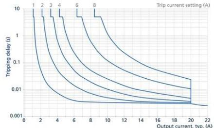
Fig. 6-2: Tripping delay depending on current
